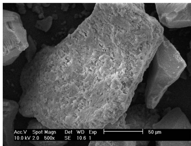
Fig. 5 Tiny particles of leach-proof and versatile catalytic ORMOSIL-entrapped perruthenate such as this 150 \mu\text{m} catalyst particle are ideally suited for being packed in capillaries and used in micro-reactions.
